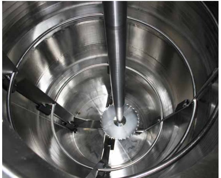
Interior view of an intensive mixer with anchor agitator and dispersion disk
