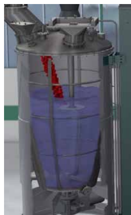
Addition of solids
