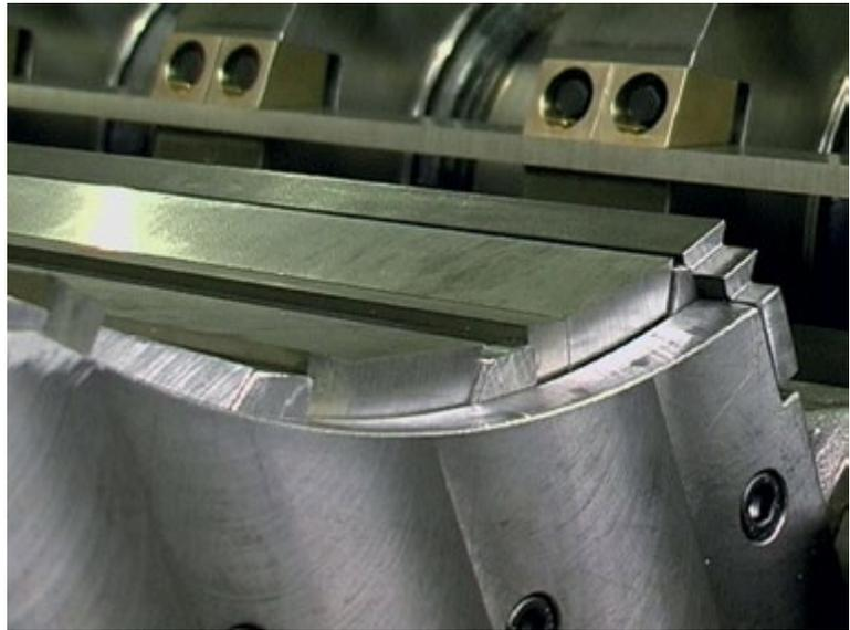
Stator knife assembly in housing side part
