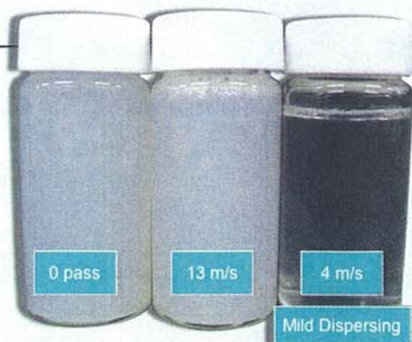
FIGURE 6. These vials illustrate the value of low agitator speeds. The unmixed solution (left) is cloudy because of particle agglomeration. Meanwhile, the vial mixed at the highest speed is also cloudy because destruction of surface characteristics causing them to reagglomerate
