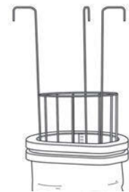
Dismounted unit (filter hose and support cage)
