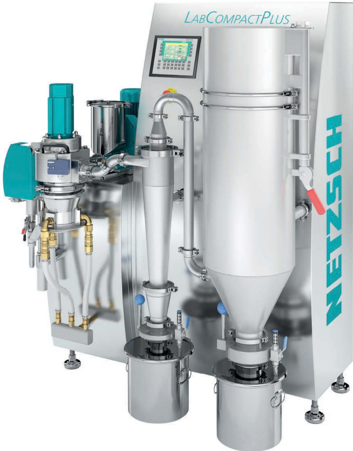
NETZSCH LABCOMPACTPLUS with Fluidized Bed Jet Mill CGS 10
