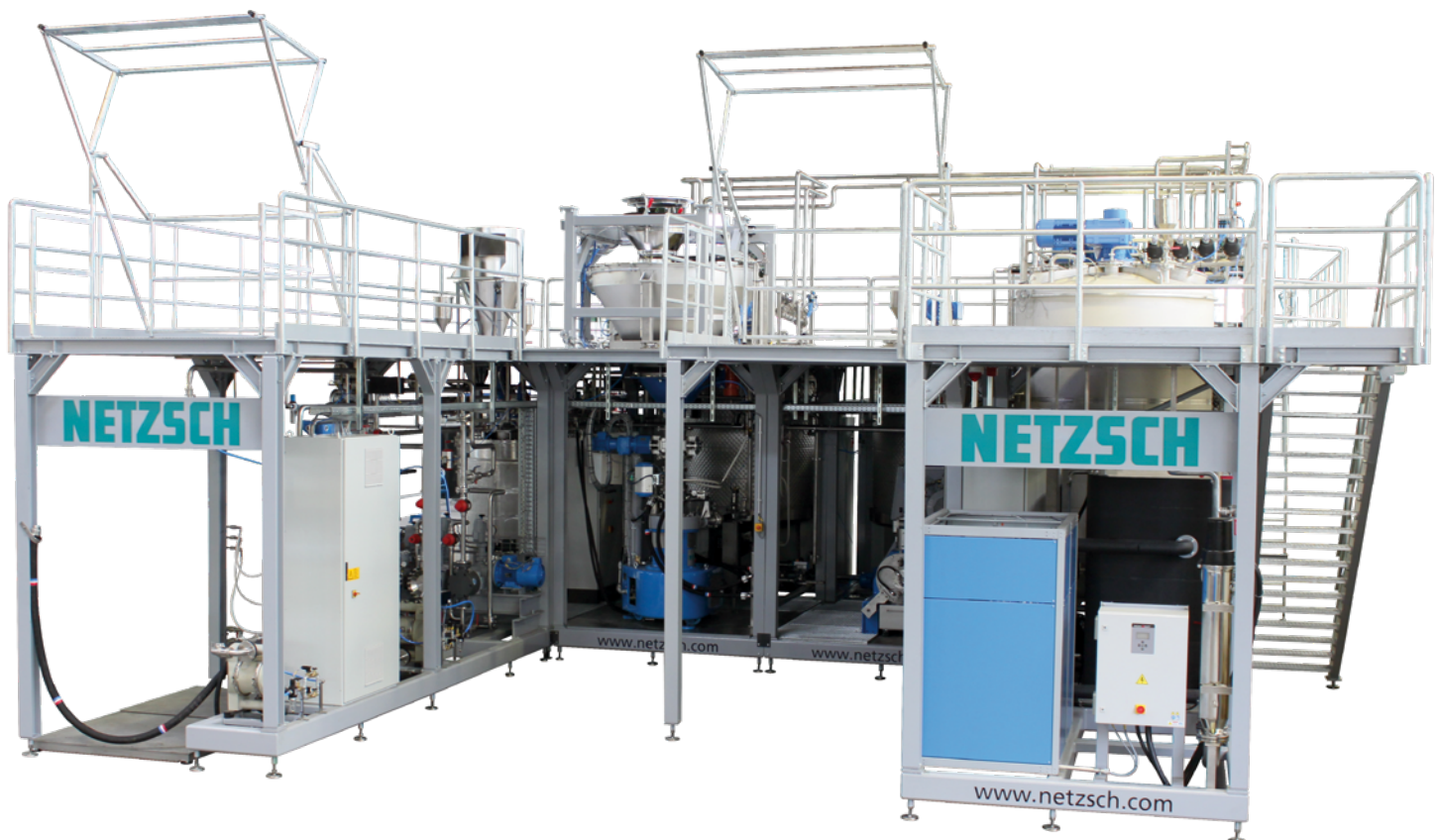
System module for seed treatment comprising: Big-Bag Feeder, Ψ-Mix ® Dispenser, ZETA ® 25 Agitator Bead Mill and modular platform
