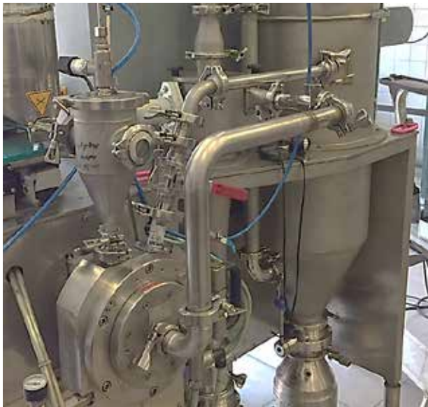
Figure 2: Laboratory plant M-JET 10 with extraction pipe in the dust filter
