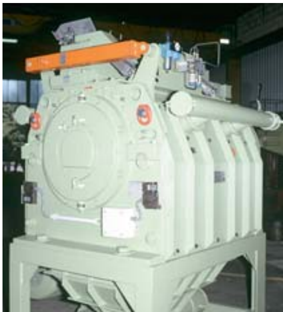
The Condux CS 500/1000-Z mill was developed for cellulose pulverisation
