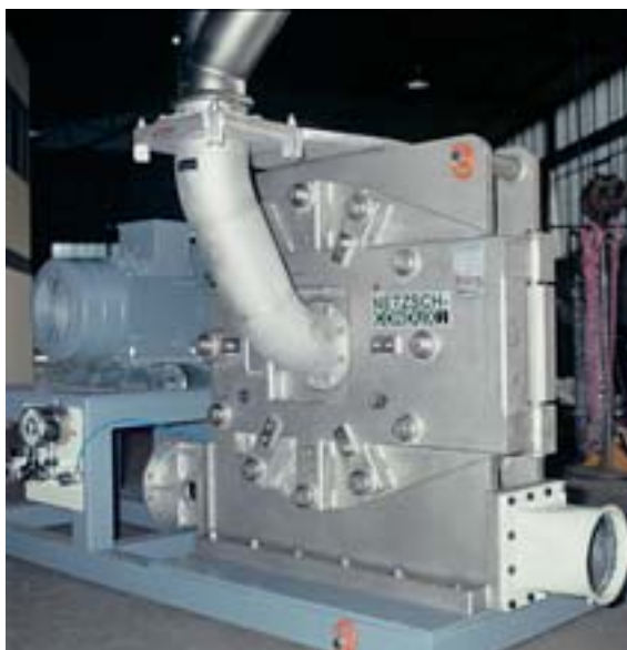
The CUM 680 universal mill can be used to fine-mill cellulose derivatives
