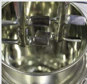
Laboratory planetary mixer Model PML 1 in vacuum design – Use of conventional, temperature-controlled tin cans as preparation containers
