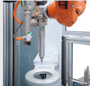
Dispenser with pressure monitoring
