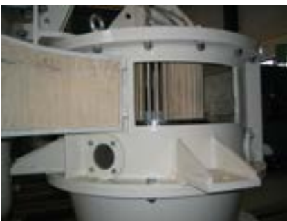
SCIROCCO 200 CD for abrasive products with ceramic flaps
