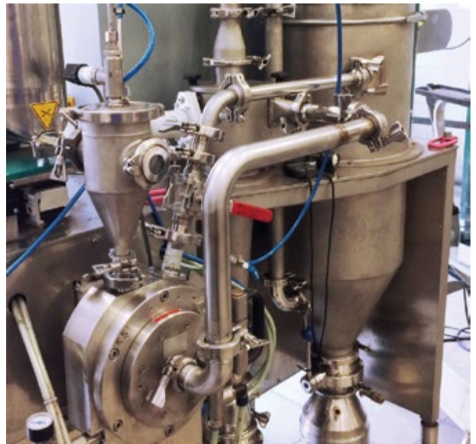
Laboratory plant M-JET 10 with extraction pipe in the dust filter
