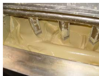
Pictures 4 and 5: Dry and wet conching with CHOCO EASY ®
