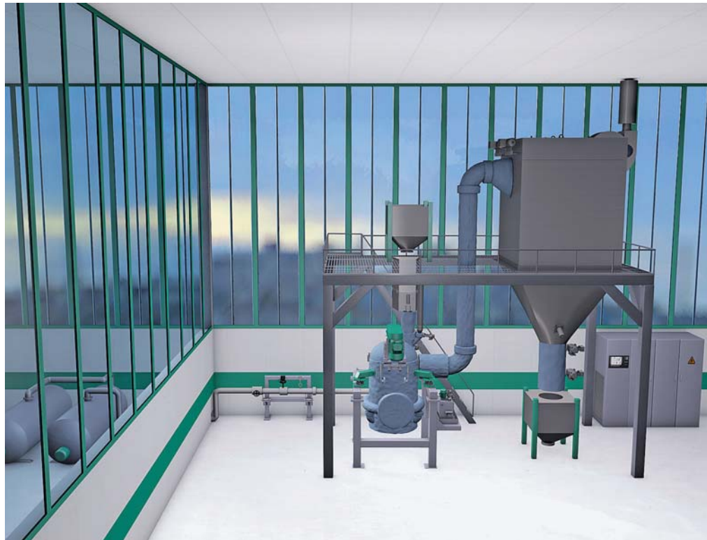
Figure 1: The s-Jet system uses superheated steam as grinding gas instead of compressed air
