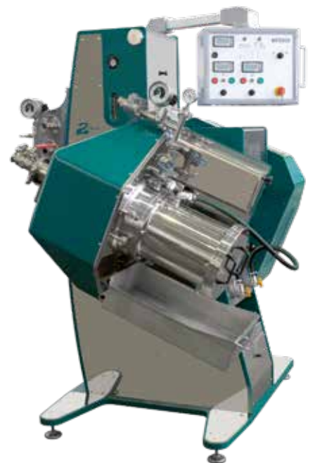
Emptying and Cleaning Position
