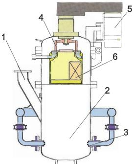
culty. The fluidised-bed jet mills in the CGS series are available in nine sizes, depending on the desired throughput. These include laboratory mills for small quantities of product up to production machines with a gas throughput of 14,000 m<sup>3</sup>/h. The CGS 10, conceived for laboratory use, uses an air flow of 50 m<sup>3</sup>/h.
