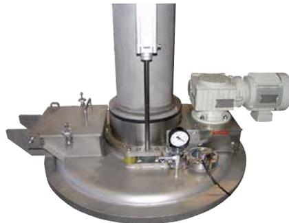
Vacuum tank cover with scraper drive
