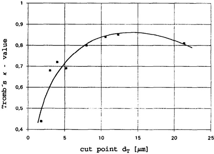
Fig. 8. Sharpness of cut as a function of the cut point for the CFS-HD classifier.
