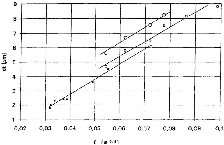
Fig. 7. Cut point of a vaned rotor as a function of the index number  $\xi$ . (○) Cylindrical rotor without immersion tube. (□) Cylindrical rotor with immersion tube. (■)  $v_{r, \text{const}}$ -rotor with immersion tube.
