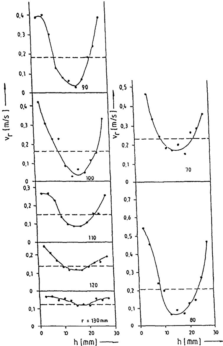
Fig. 5. Radial velocity profile in the vane-free internal area of a cylindrical rotor.
