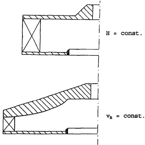
Fig. 6. Schematic view of a cylindrical rotor (top) and a rotor of theoretically constant radial velocity (bottom).
