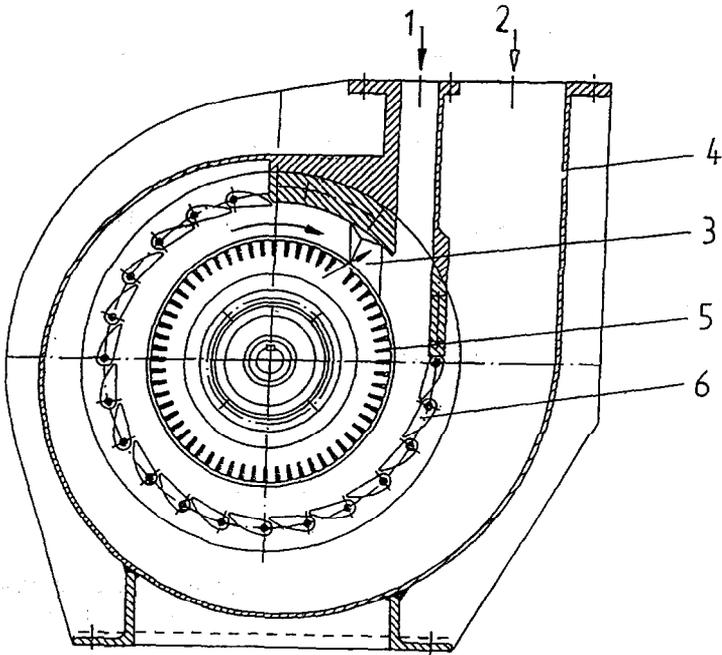
Fig. 3. Schematic drawing of the CFS-HD classifier. 1: Product feed; 2: Air inlet; 3: Coarse fraction discharge; 4: Housing; 5: Rotor; 6: Static vanes.
