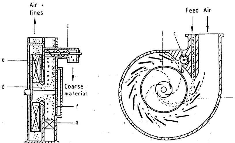
Fig. 1. Free vortex classifier Alpine Mikroplex. (a) Adjustable guide vanes; (b, c) coarse fraction discharge; (d) fines outlet; (e) fan; (f) rotating walls.
