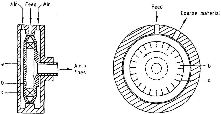
Fig. 2. Deflector wheel classifier Donaldson Acucut. (a) Housing; (b) rotor; (c) vanes.
