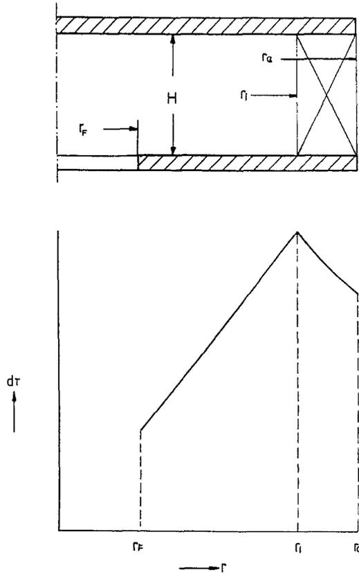
Fig. 4. Qualitative graph of the cut point versus the radius in a vaned classifier rotor.
