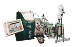
The *LabStar* designed in protection class IP or Ex has an electrical drive of 3 kW which is infinitely adjustable via frequency inverter. Depending on the grinding system, the grinding chamber volume is between 0.6 – 0.75 l. Product batches of 1.5 – 5 l can be processed. The laboratory mill can be operated with the well-known
