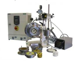
The MINICER and MINIPUR have a peg agitator, however, contrary to the MINIZETA, both machines work with the highly-efficient rotor slotted pipe centrifugal system. This enables the use of small grinding media of 0.3-2 mm in diameter. The ceramic coolable grinding tank also allows a discontinuous operation whereby the product inlet and outlet can be closed with a blind plug.
