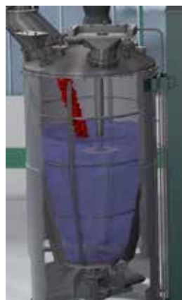
Addition of solids
