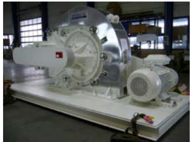
SIERRA 63 special design: Heart insulated for coating of \text{CaCO}_3 with stearic acid
