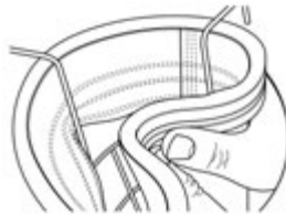
Mounting of the filter hose with snap ring
