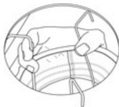
Hooking of the unit onto the perforated filter plate
