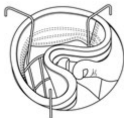
Dismounting of the filter hose with snap ring
