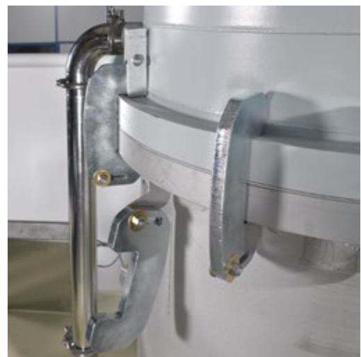
Easy loosening of clamping brackets without tools in relieved state
