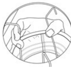
Unit is hooked off by pushing together the springs
